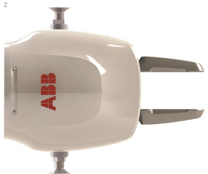
1. Servo gripper (hand) and one pneumatic, with camera | 2. Servo gripper (hand) and two pneumatics with status lights
