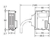
● 8/6-point Basic I/O Units, Interrupt Input Unit, and Highspeed Input Unit
