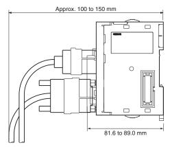
Note: Consider the following points when expanding the configuration: The total length of I/O Connecting Cable must not exceed 12 m. I/O Connecting Cables require the bending radius indicated below.
