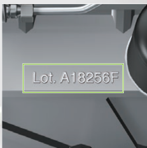
Presence inspection of marked characters
