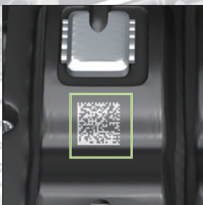
Reading direct part marks
