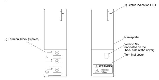
Note: In the left side figure, the terminal cover is removed only for explanation purpose. The right side figure shows the terminal cover mounted condition.
