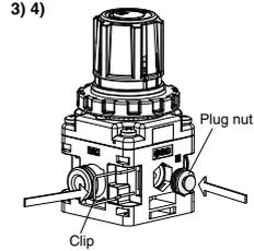
Note) To remove the pressure gauge or pressure switch, remove the clip, then remove the pressure gauge or pressure switch straight out. Do not apply torque, as the body is made of resin.
