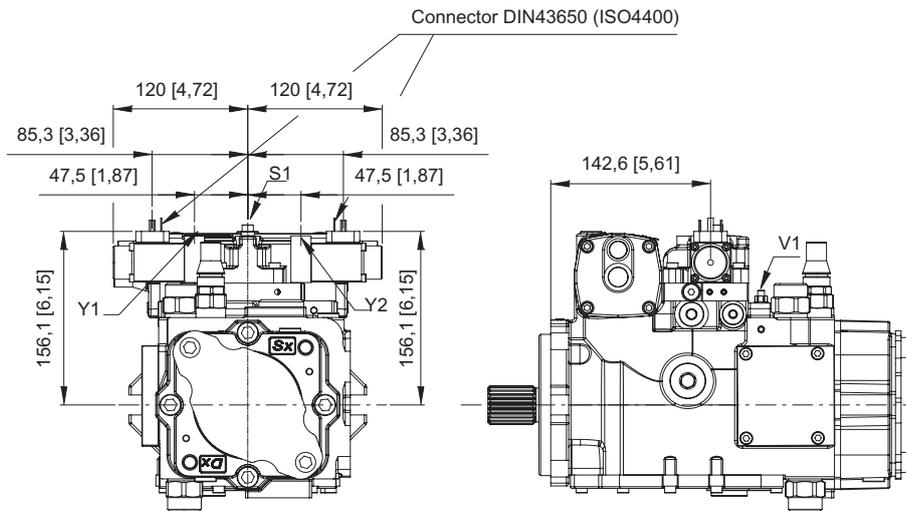
Y1-Y2: Attacchi pilotaggio comando / control piloting pressure ports - 1/8" G (BSPP) (ISO)
