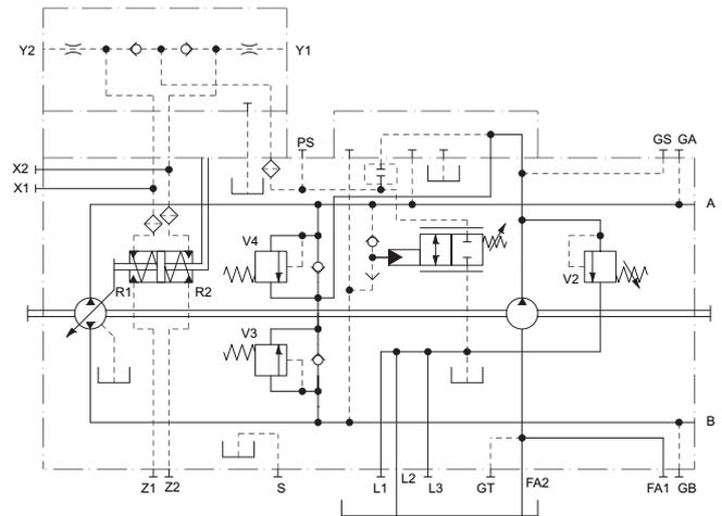
Pilot pressure = 6÷14 bar [87÷203 psi](at ports Y1, Y2)
