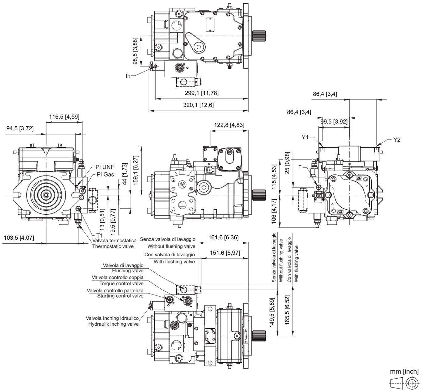
Y1-Y2: Attacchi pilotaggio comando / Control piloting pressure ports - 1/4 G (BSPP) (ISO)
