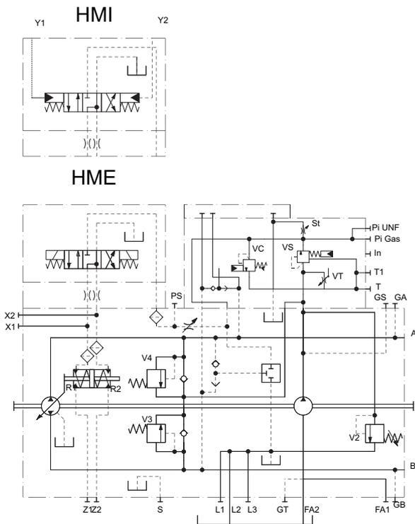
The "AUTOMOTIVE" (speed related) control, is used in hydrostatic transmissions with closed loop variable displacement pumps.
