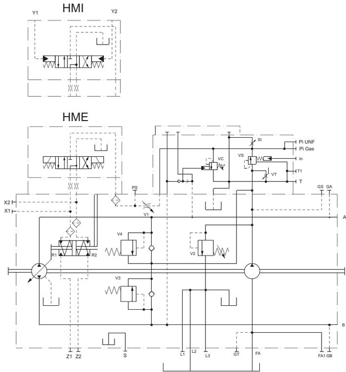
The "AUTOMOTIVE" (speed related) control, is used in hydrostatic transmissions with closed loop variable displacement pumps.
