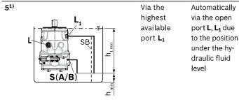
A check valve in the drain line is only permissible in isolated cases. Consult us for approval.
