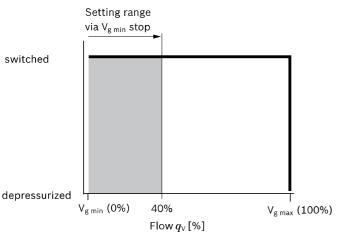
$\begin{array}{cccc} \text{Depressurized} & \triangleq & \text{$V_{g\,\,max}$} \\ \text{Pressure switch on} & \triangleq & \text{$V_{g\,\,min}$} \end{array}$
