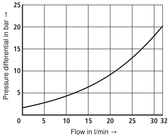
\Delta p - q_v -characteristic curve via the check valve (B → A) Orifice closed
