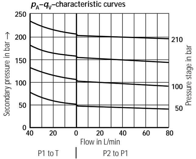
**⚠ Attention!** The curve characteristics are maintained at lower set pressure in relation to the pressure stage.
