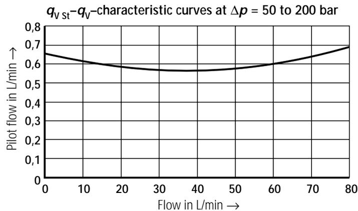
The characteristic curves for the pressure reducing function are valid for an output pressure = zero in the entire flow range!
