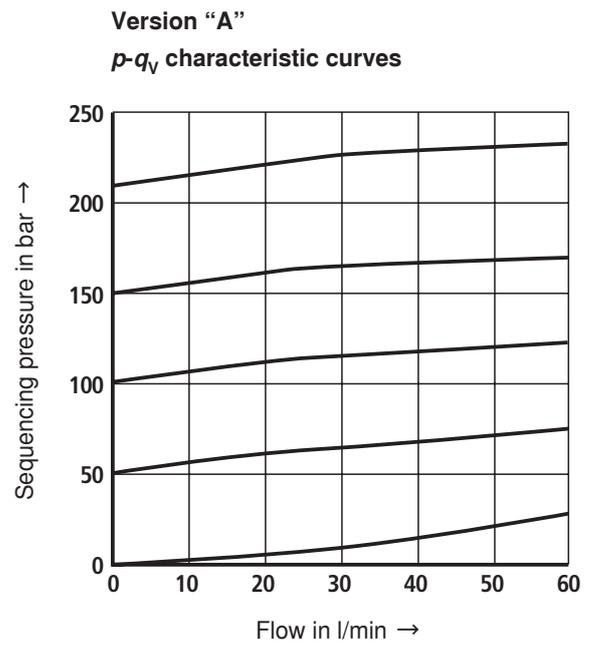
The characteristic curves apply to initial pressure = zero in the entire flow range!
